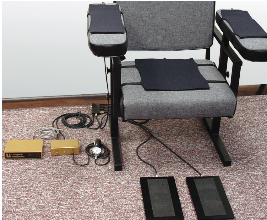
Figure 2. Lafayette 76875S Activity Sensors configured with polygraph testing chair. Photo courtesy of the Lafayette Instrument Company, Inc.
